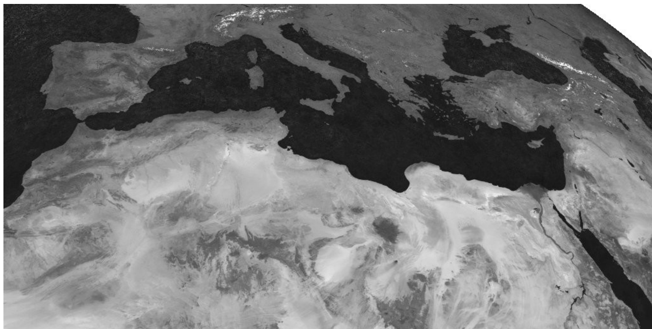
MFG: 1995-2005, 2.5 \times 2.5 \text{ km}^2 resolution at sub satellite point, 2 images per hour
